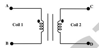
The figure above shows coils 1 and 2, with dot markings as shown, having 4000 and 6000 turns respectively. Both the coils have a rated current of 25A. Coil 1 is excited with single phase, 400V, 50Hz supply
