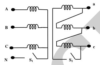
The star-delta transformer shown above is excited on the star side with a balanced, 4-wire, 3-phase, sinusoidal voltage supply of rated magnitude. The transformer is under no load condition.
