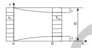
The velocity profile is uniform with a value of  $u_0$ at the inlet section A. The velocity profile at section B downstream is
