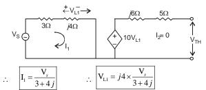
\*  $V_{TH} = 10V_{11}$  because no-current flowing through circuit.
