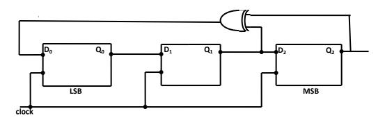
Which one of the following is the correct state sequence of the circuit?
