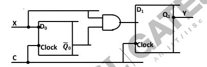
Consider the following timing diagrams of X and C; the clock period of  $C \ge 40$  nanosecond. Which one is the correct plot of Y?
